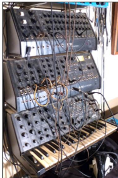
Most importantly it also features two voltage-controlled filters – low pass and high pass, 12dB roll-off. Both filters go into self-oscillation with high resonance settings. This is, I believe, at the heart of what makes this synth produce such unique sounds!
